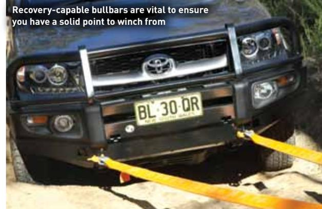
Recovery-capable bullbars are vital to ensure you have a solid point to winch from
